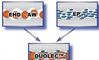
EHD and mixed film antiwear components of DUOLEC™ kick in. After loads become even greater, then the boundary lubrication extreme pressure performance of DUOLEC™ is activated.
