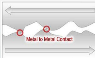
Figure 1: Asperities on touching metal surfaces
